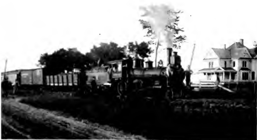
This is the only surviving photo of the second M&WI steam engine numbered 1, a 4-4-0. It is posed, probably in the 1905-1908 period, with a mixed train consisting of a gondola, boxcar and combine 1 southbound at the Darius Runkle house just north of Littleton. This large house, built in 1866, was still standing in 2005. Image courtesy of the Schuyler County Jail Museum
