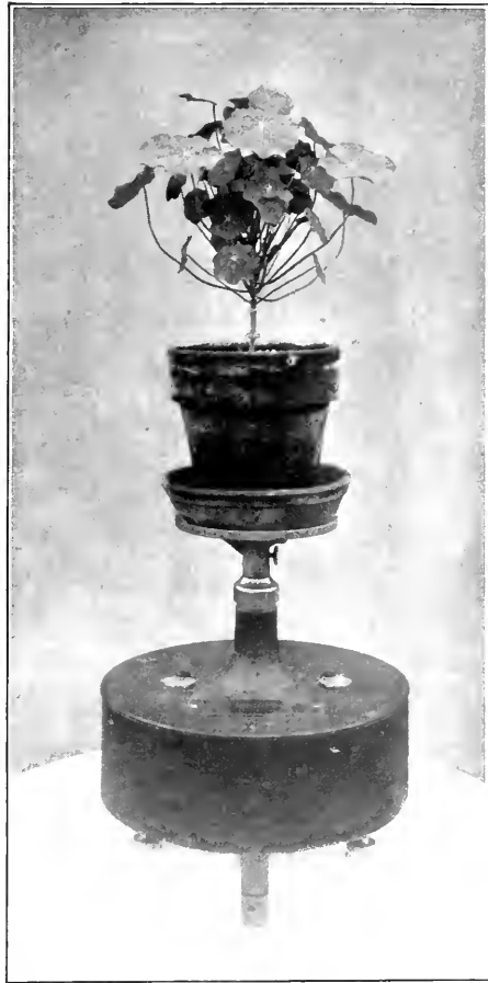
FIG. 83.—The clinostat, an instrument which allows the effect of one-sided stimuli to be neutralized through the continual slow rotation of the plant. Note the resultant symmetry of the Nasturtium which has been grown from seed on the instrument.
