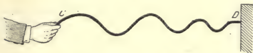
FIG. 22.—A cord is fixed at one end D , and if the other end C , held in the hand, is moved briskly up and down, a serpentine movement is produced which will give an idea of the undulatory movement of Fig. 21 if we regard it for instance as following the ray OX .
