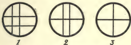
FIG. 42.—Diagrams 1, 2, and 3 show the aspects under which the crossed metal wires should appear successively on the small fluorescent screen, when a tube is centred by means of a centring device with crossed wires.
