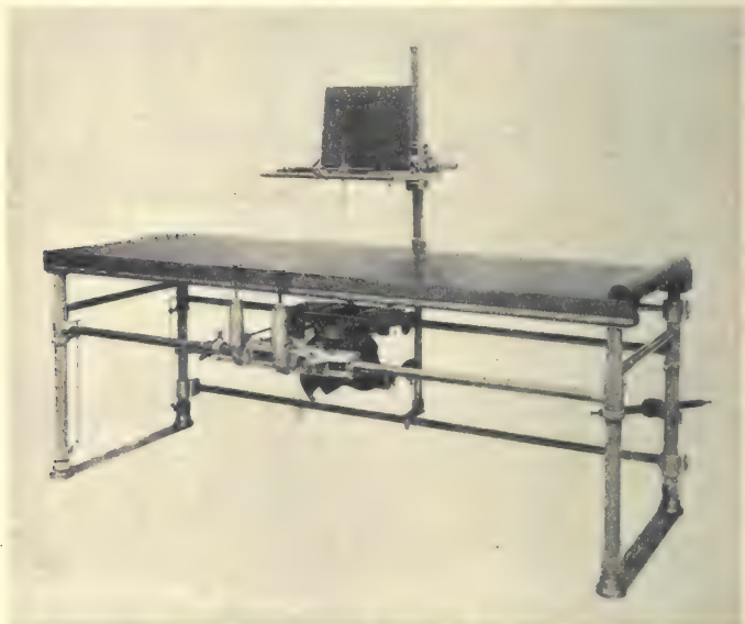
FIG. 68.—X-ray surgical table by Dr. R. Ledoux-Lebard (Gallot & Co.) made entirely of metal. Its height is adjustable by means of a bayonet arrangement in its legs. The height can thus be adjusted as required to suit the height of the surgeon, or if only one side is lifted it can be inclined as much as is desired for abdominal explorations.
