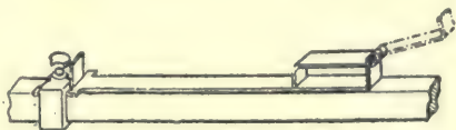
FIG. 141.—The stop device of the skiameter. It allows a displacement of five centimeters on each side of the normal ray.
