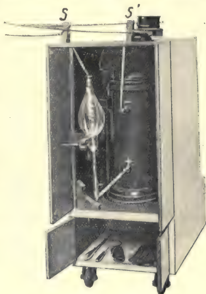
FIG. 59.—In order to use the apparatus all that is required is to pull out the holder which carries the valve and to lift out the spintermeter and milliampère-meter. All that remains now is to connect the tube to the extremities S and S' of the spintermeter. The small lower compartment containing the various accessories is shown closed in Fig. 58 and open in Fig. 59 in which we can see the various accessories (such as gloves, spectacles, pointers, ink marker).
