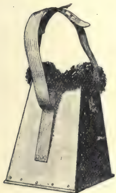
FIG. 73.—Radioscopic X-ray screen and fluoroscope by Dr. Réchou (Gallot & Co.).
