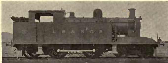
4-4-2 TYPE PASSENGER TANK LOCOMOTIVE L.B. & S.C.R.
