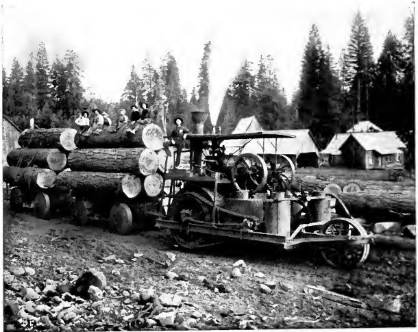
FIG. 51. — A Holt Three-wheeled Traction Engine hauling Sugar Pine Logs. California.
