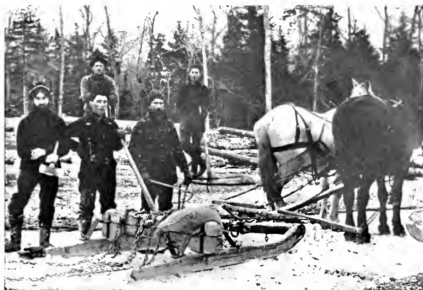
FIG. 34. — A Yarding Sled used in the Northeast.
