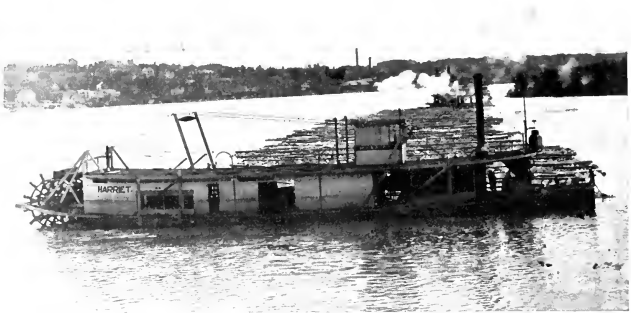
FIG. 115. — A Mississippi River Log Raft, showing the Method of Control by End-wheel Steamers.
