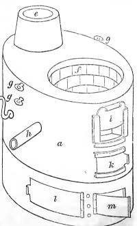
half an inch deep. The ash-pit is furnished with a door, m, which opens on hinges, intended for removing the ashes;
