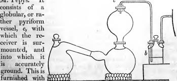
a glass valve, which allows gas to pass freely into it from the receiver, but prevents the water which it contains from falling into the receiver. From this a common tube rises, to connect the tubulated receiver, b, as in the former apparatus.
