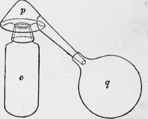
these kinds of apparatus, acids, and other substances which arise from chymical decompositions, aided by heat, are distilled; and the process is named distillation *per latus*; but if the products be highly volatile, or of a gaseous nature, the pneumato-chymical apparatus, to be afterwards described, is required. For the preparation of alcohol, and of distilled waters, the common still is employed. It consists of two parts-the
