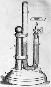
a quarter of an inch below the cork. A piece of glass rod, an inch long, is then to be put into the short leg, and afterwards a piece of sheet zinc bent double, which will fall down until stopped by the glass rod. The stopcock being then inserted and left open, in a few minutes the gas that issues should be lighted. If arsenious acid be present, metallic arsenic and a circle of oxide will be formed on the piece of glass, f, held over the flame.
