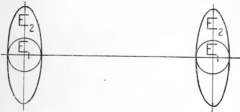
Fig. 5.—Representing the meridian section of two coaxial electrons, the charge in the inscribed sphere being electrostatically equivalent to a point, and of the rest equivalent to a ring.
