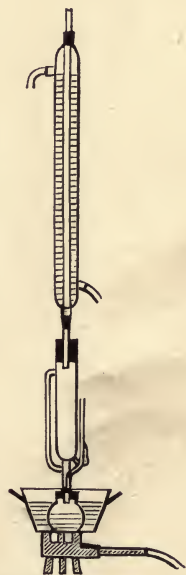
FIG. 64. Fat Extraction Apparatus.
