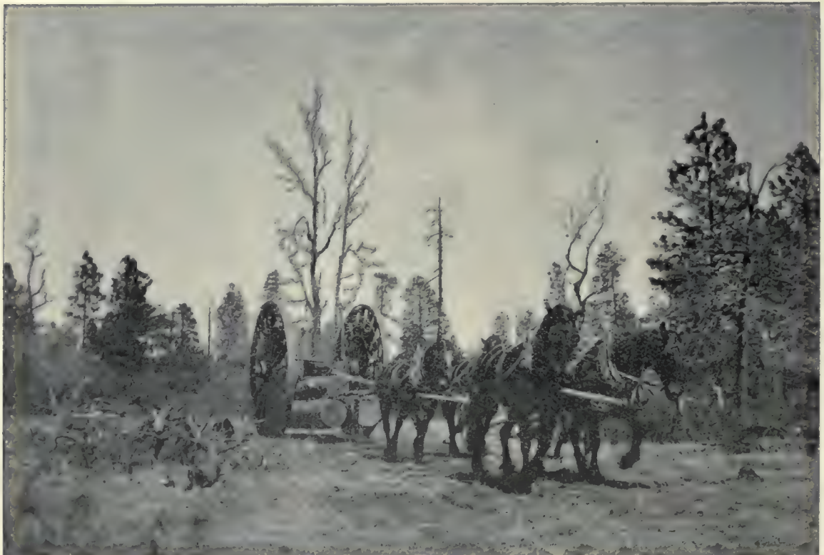
(2). Same as above ; 4 horses hauling 3 tons of logs on fairly level but rough ground.—Flagstaff, Arizona.
