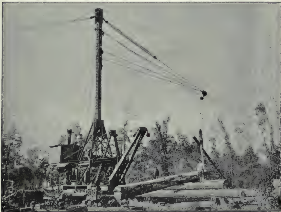
(2). Lidgerwood Overhead Skidder, lowering steel spar type, with swinging loading boom.
