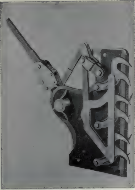
(1). Usual type of board Dog, one face of the knee removed.
