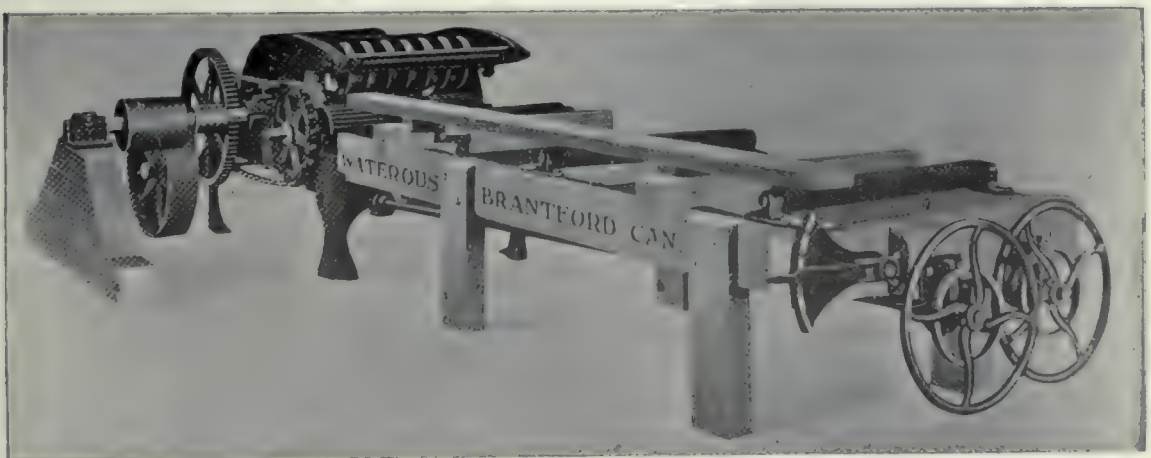
(2). A 30 inch Double Edger. (By permission of Messrs. The Waterous Engine Works Co.)
