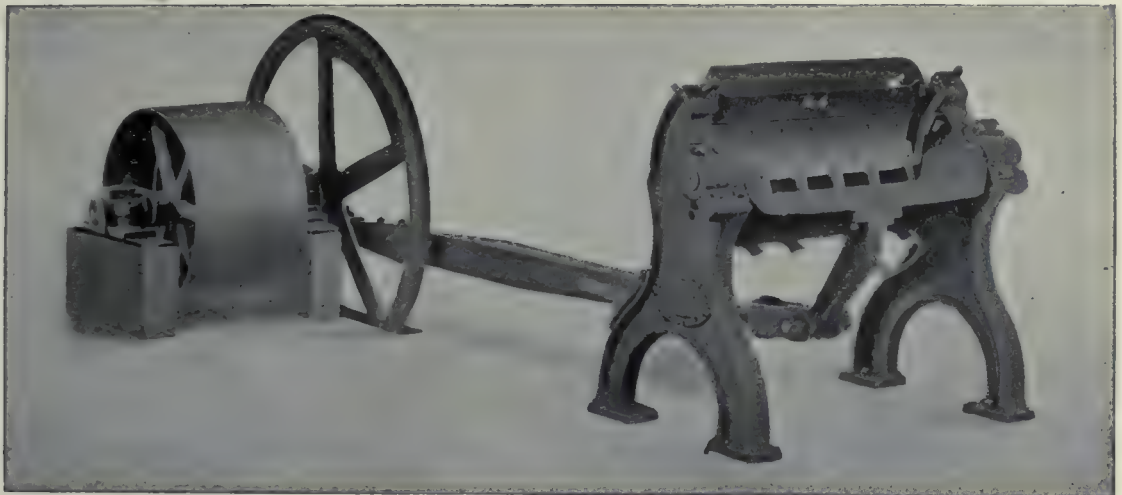
(1). Stave Cutting Machine. (By permission of Messrs. The Rochester Barrel Machine Co.).
