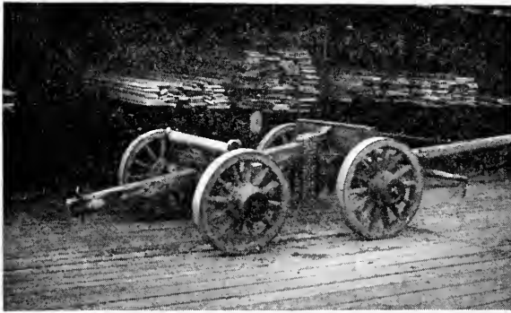
FIG. 107.—A Wagon with a Rear Roller used in hauling Lumber from the Assorting Table to the Yards. The view shows the Wagon short coupled for ease in hauling it when empty.
