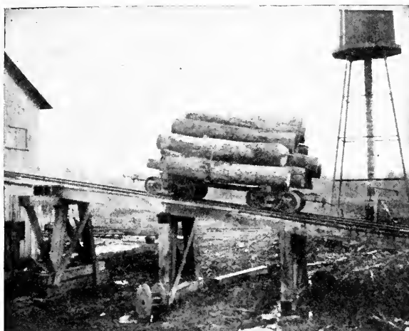
FIG. 13.—A Loaded Log Car going up the Incline leading to the Sawing Floor. A Method used at some Plants which do not have Log-storage Facilities.
