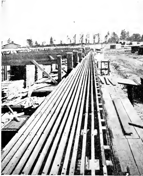
FIG. 102.—The Terminus of an Edge Sorter showing Storage Pockets on the Left.
