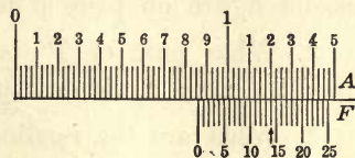
PART OF THE SCALE OF A VERNIER CALIPER
