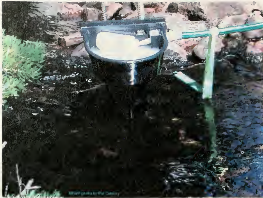
Figure 14. Close-up view of the dog waterer trickling CFT/streamwater mixture into the stream during the Cherry Creek Project.
