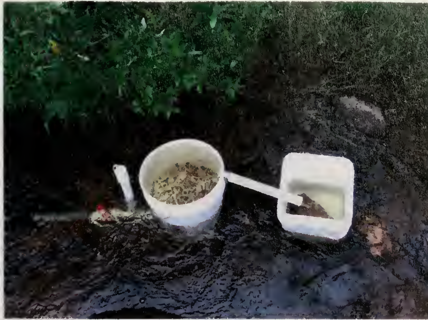
Figure 15. Remote streamside incubator (round bucket) and capture bucket (square bucket) in Cherry Creek
