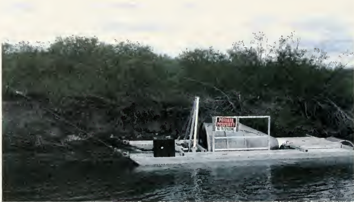
Figure 53. Rotary screw trap typically used to sample young-of-the-year and yearling fish on Hebgen tributaries.
