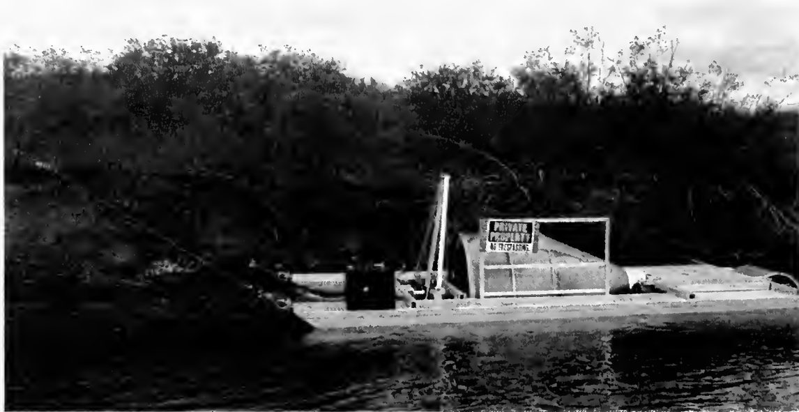
Figure 53. Rotary screw trap typically used to sample young-of-the-year and yearling fish on Hebgen tributaries.
