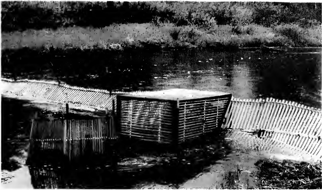
Figure 25. Rigid weir assembly used to trap immigrating rainbow trout on Duck Creek and the South Fork Madison. MFWP photo by Travis Lohrenz.
