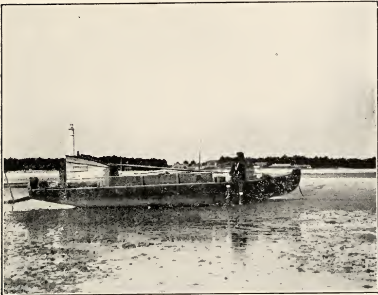
FIG. 8.—HOPPER BARGE USED FOR THE REMOVAL OF SAND, CAPE FERRET OYSTER PARKS.
