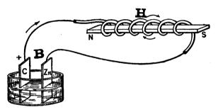
FIG. 18.-VOLTAIC CELL SUPPLYING CURRENT TO A HELIX. magnetic flux issues from and enters into the iron.
