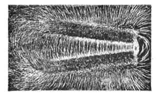
FIG. 19.-MAGNETIC FLUX OF HORSESHOE MAGNET. representing the direction of the flux lines in the plane of the glass plate.
