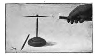
FIG. 3.—ATTRACTION BETWEEN ONE POLE OF A PIVOTED NEEDLE, AND THE POLE OF THE APPROACHED BAR MAGNET. of the Northern Hemisphere the needle will come to rest with its north pole pointing approximately to the earth's geographical north? The reason may be
