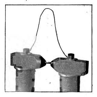
FIG. 73.—PARAMAGNETIC SUBSTANCE BETWEEN MAGNET Poles.
