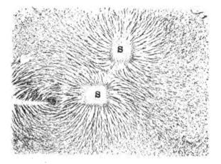
FIG. 24.—FLUX PATHS. LIKE POLES AT RIGHT ANGLES.
