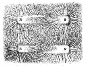
FIG. 21.—FLUX PATHS OF TWO ADJACENT BAR MAGNETS. sentations of groupings of filings obtained by either of the above described processes cannot be regarded as marking accurately the exact flux paths; since, in reality,
