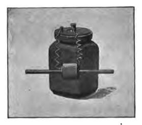
FIG. 40.—ELECTROMAGNETIC EFFECT OF AN ELECTRIC CUR-RENT PASSING THROUGH A COIL OF WIRE.
