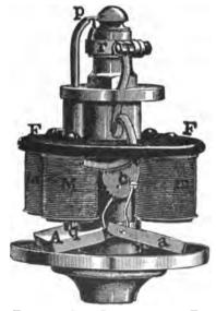
FIG. 61.—ELECTRIC GAS LIGHTING AND EXTINGUISHING MECHANISM. sage of a current through the coils, and the contact of the platinum-tipped wire p, with the projection on the ring r,
