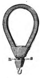
FIG. 49.—COMPOUND PERMANENT MAGNET WITH CONSTANT POLE SURFACES.
