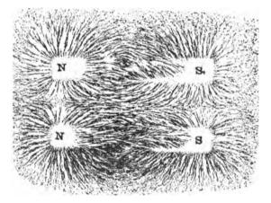
FIG. 22.—FLUX PATHS OF TWO ADJACENT BAB MAGNETS, of the flux lines which occurs inside the body of the magnet.
