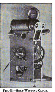
net at the base FIG. 63.—SELF-WINDING CLOCK. of the clockwork receives a brief electric current, say every fifteen minutes, and at-
