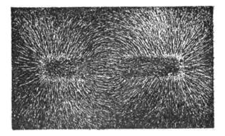
FIG. 15.—FLUX OF BAR MAGNET.
