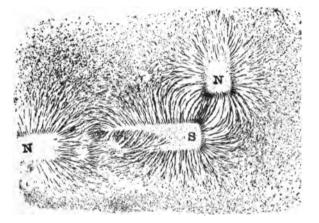
FIG. 23.—FLUX PATHS. UNLIKE POLES AT RIGHT ANGLES. one magnet is adjacent to the north pole of the other magnet. The flux streams passing out of the north pole of each magnet enter the south pole of the adjacent magnet, the flux from one magnet merg-
