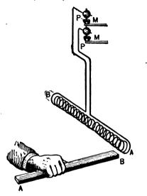
FIG. 35.-HELIX CONVEYING AN ELECTRIC CURRENT POS-SESSING MAGNETIC PROPERTIES.
