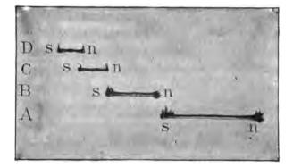
FIG. 9.—POLARITY OF DISSECTED MAGNET.
