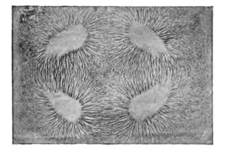
FIG. 28.—FLUX PATHS OF TWO SEMICIRCULAR BAR MAGNETS. at the centre of the figure, and at this point there would be little or no directive tendency exerted upon a very small compass needle.
