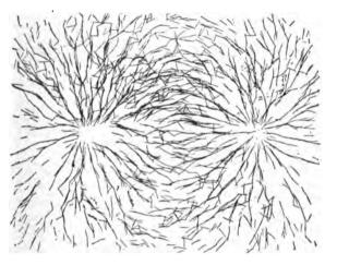
FIG. 25.-FLUX PATHS OF BAR MAGNET. IRON WIRES.
