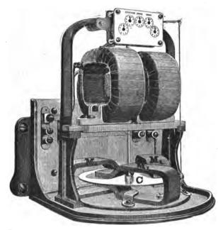
FIG. 78.—RECORDING WATTMETER WITH MAGNETIC BRAKE. magnetic field, has received a number of practical applications in the arts. One of
