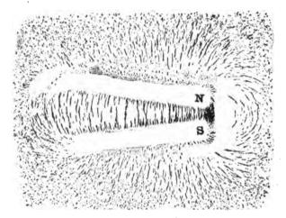
FIG. 20.—FLUX PATHS OF TWO ADJACENT BAR MAGNETS. pears destitute of flux paths. This, however, is due to the fact that on tapping the glass plate the powerful attraction of the poles for the magnetized particles has caused them to here slide over the smooth surface of the glass and collect between the poles.
