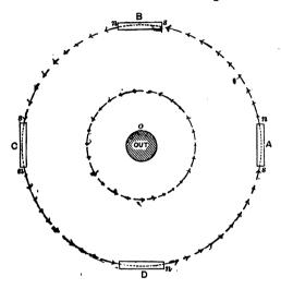
FIG. 31.—DIRECTIVE INFLUENCE OF CIRCULAR MAGNETIC FLUX AROUND ACTIVE CONDUCTOR CARRYING CURRENT TOWARD OBSERVER.
