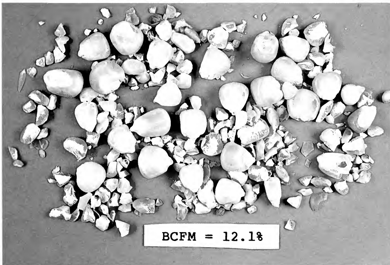
Loading of the ocean vessel caused breakage when stress-cracked kernels impacted the spouting.
