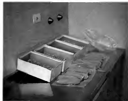
Samples of flint maize taken from farmers' fields, combines, and trucks were air-dried immediately to prevent deterioration and minimize the development of stress cracks.
