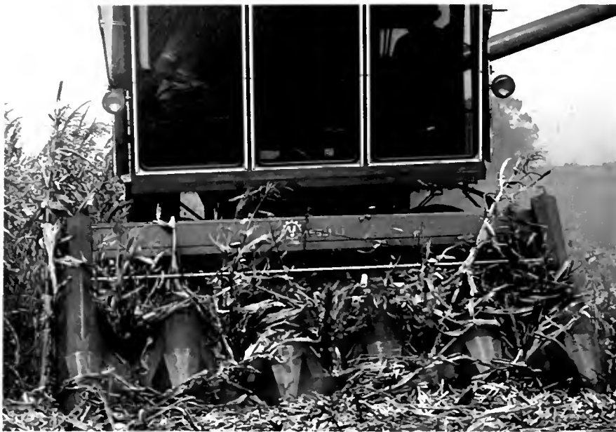
Harvesting maize in Argentina is a fully mechanized operation, as shown by this Vassalli combine with a 5-row Manerio header.
