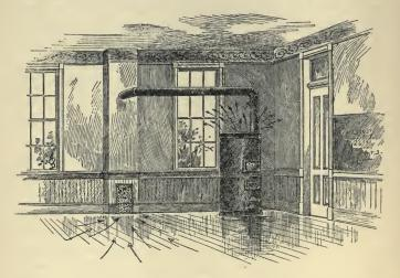
sheet-iron division is, however, not necessary, since the ventilating duct can open, as above stated, directly into the chimney shaft, if it be made secure against fire at the floor.
