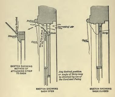
ble, by placing a strip of tin or rubber, or even pasteboard, on the upper edge of the lower window sash, so adjusted as to touch the panes of glass in the upper window sash.
