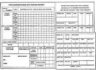
FORMS 4, 5, 6: In front at the right is Form 4 used by the time-keeper as the basis of all his reports. Form 5 at the left, a semi-pay period report on each man's earning power is made out from the remaining, coupon (Form 6) which is one variety of the several similar work tickets used by different departments
