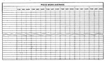
FORM 11: The top spaces on this form are for operatives' numbers. The spaces at the left are for pay period dates. In the columns are entered the total time, total pieces and the worker's average output per hour
