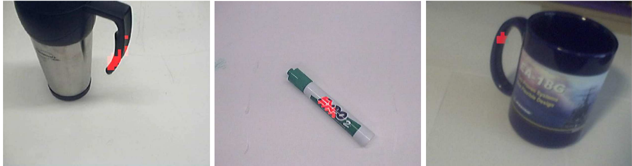
Fig. 3. Grasping point classification. The red points show the predicted grasping point.
