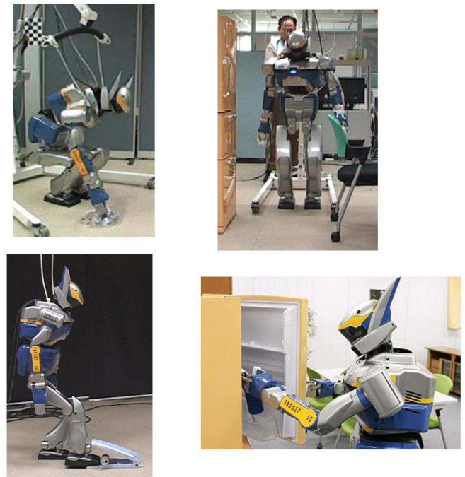
Fig. 8. Various Tasks Realized using the Proposed Operation System
