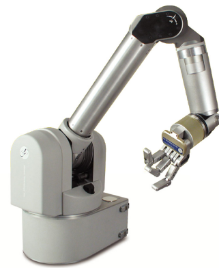
Fig. 5. Barrett Technologies Whole Arm Manipulator (WAM)
