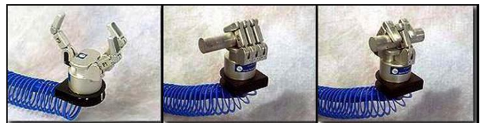
Fig. 6. Barrett Technologies three-fingered hand
