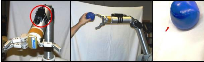
Fig. 8. Visual servoing: Sony XCD710CR camera mounted on UMan ’s wrist, UMan ’s arm tracking the blue ball in an attempt to center it in the image plane, the velocity vector commanded by the vision system
