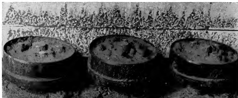
FIG. 40. After 75 minutes of artificial rain, the splash erosion is clearly evident. The white board behind the pots is six inches away. On sloping land, the splashed soil would fall into the surface flow of water and be carried downhill. The coins illustrate the protective nature of mulch.
