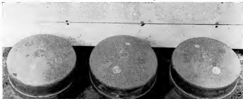
FIG. 39. Three soil samples with coins placed on surface. The setup is similar to a well prepared seedbed.
