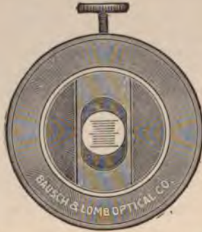
Fig. 12.—Micrometer Eyepiece Viewed from Below.
