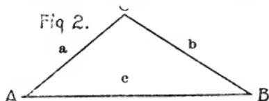
4. Prove that the area of any plane triangle is equal to half the rectangle of any two sides multiplied by the sine of their included angle.
