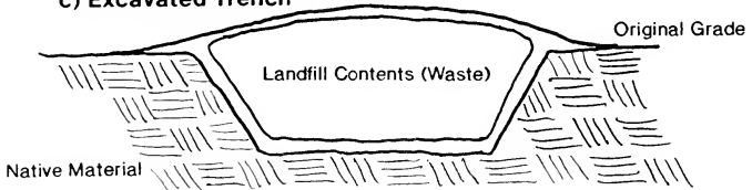
c) Excavated Trench
