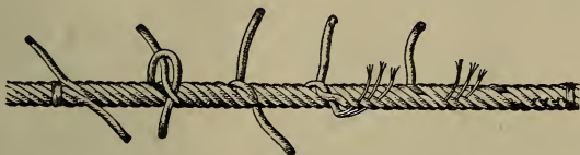
Fig. 2 1 st Method Long Splice in Wire Rope. (2)
