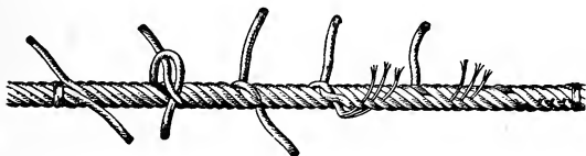
Fig. 2 1 st Method Long Splice in Wire Rope. (2)
