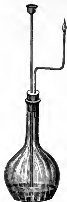
Student's apparatus for making arsenic spots.
