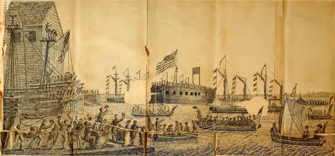
LAUNCH OF THE STEAM FRIGATE FULTON THE FIRST, AT NEW YORK 29 TH OCT. 1814. 150 feet long and 37 feet wide, will mount 30 long 32 pounders, and 2 700 pounders (Columbiads)
