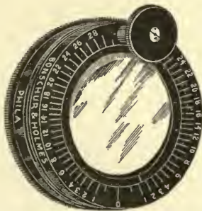
FIG. 85.—Rotary variable prism.
