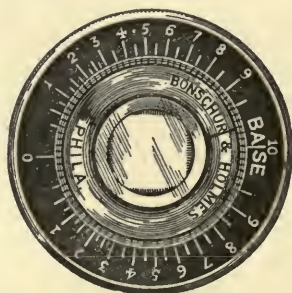
FIG. 84.—Phorometer combining Maddox rod and rotary prism.
