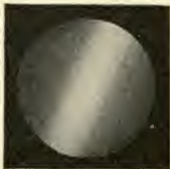
FIG. 73.—Band-like appearance in direction of principal meridian of greatest curvature at 70°.
