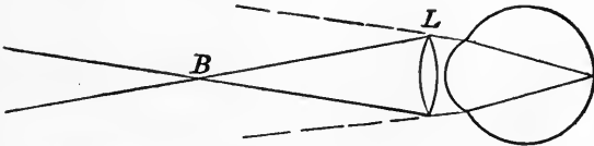
FIG. 59.—Rays emerging from a hyperopic eye rendered convergent to give a point of reversal.
