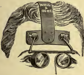
FIG. 21.—Binocular magnifier supported by a spring steel headband, for examination of the eye, and the performance of certain operations.
