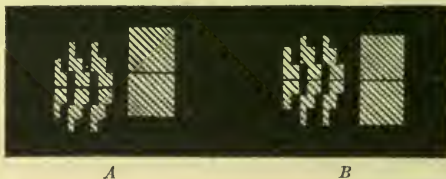
FIG. 71.—Mires of the ophthalmometer: A , with the arm not corresponding to either principal meridian of the cornea; B , turned to one of the principal meridians.
