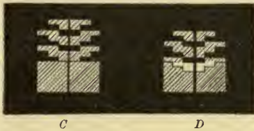
FIG. 72.—Mires of the ophthalmometer: C , in the meridian of least refraction, just touching; D , in the meridian of greatest refraction, overlapping for 1.75 D. of astigmatism.
