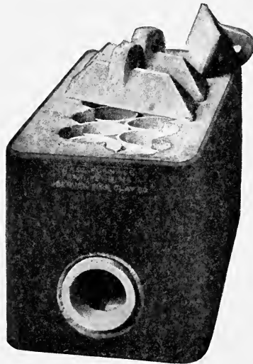
FIG. 12. — GASOLENE-BURNING CRUCIBLE FURNACE
