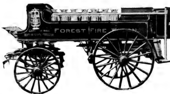
Fig. 59. — Special forest fire wagon; large size for two horses.
