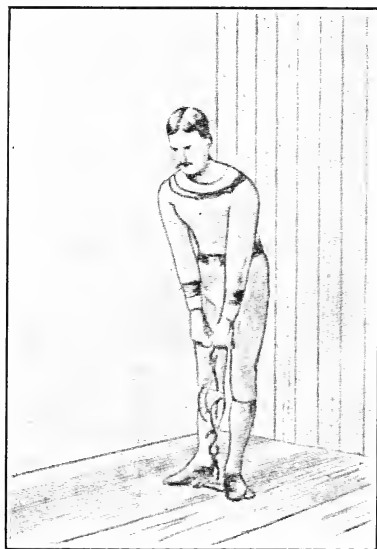
FIG. 18. BACK AND LEG DYNAMOMETER, AS USED FOR STRENGTH OF BACK.
