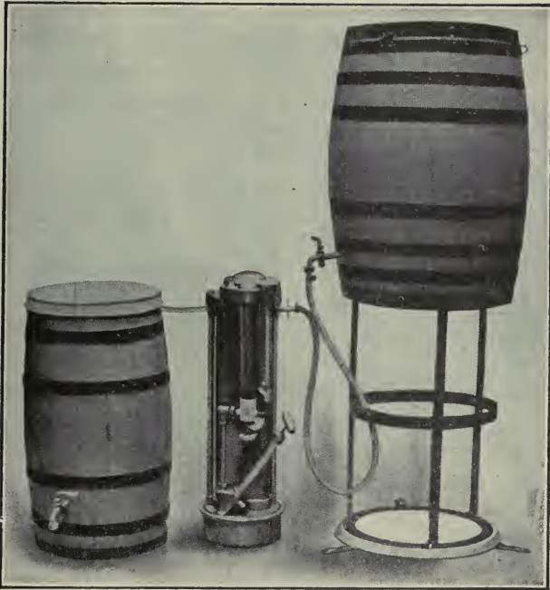
FIG. 46.—Barrel accessory set up, ready for operation in connection with the Forbes sterilizer.
