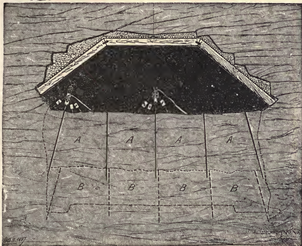
FIG. 309.—Drilling Bench-holes in the American System of Tunnelling.
