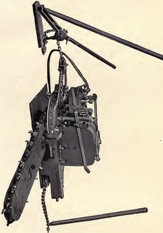
Fig. 318.—The Sullivan Coal-cutter.
