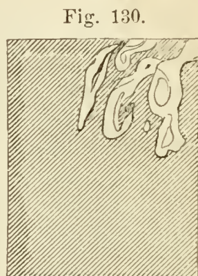
“Marbled” or “oyster-shell” surface stains.
