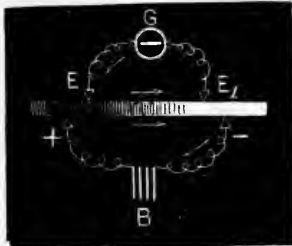
Fig. 302.—Diagram to show Distribution of 'Positive Polarization' after opening Polarizing Current. B, battery; G, galvanometer. The dark shading signifies that the excitation to which the current causing the positive deflection after the opening of the polarizing current is due is greatest in the immediate neighbourhood of the anode, and fades away in the intrapolar region. + indicates the anode, and - the kathode of the polarizing current.
