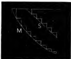
Fig. 243—Curves of Extensibility. M, of muscle; S, of an ordinary inorganic solid.
