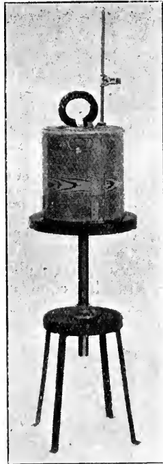
Fig. 51.—Calorimeter with stand for measuring blood-flow in hand.
