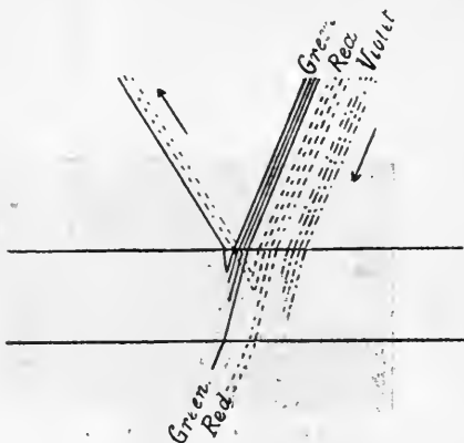
Fig. 415.—Diagram to show Connection of Body Colour with Selective Absorption.
