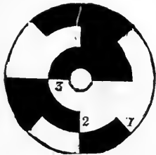
Fig. 446.—Disc for demonstrating Talbot's law.
