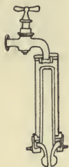
Sectional view of 56, A, showing relation of parts with filtering "bougie" in position.
