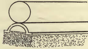
DRAIN AND SUBSOIL PIPE LAID UPON CRUSHED STONES.
