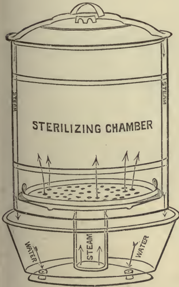
FIRST FORM OF ARNOLD'S STEAM STERILIZER. Tall, narrow, disinfecting chamber.
