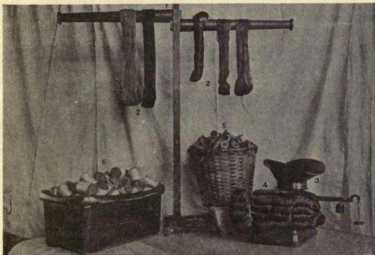
FIG. 4.—1. Skein parting and dressing pole. 2. Roll, and skein, of yarn. 3. Scale for weighing yarn. 4. Bundle of dyed silk yarn. 5. Mill basket, with empty bobbins. 6. Fibre mill box with wound bobbins.
