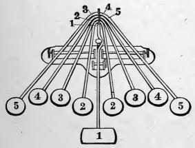
From the accompanying cut it will be seen that there are only five keys, although at first sight there appear to be more. No. 1 is straight and has a marker on the end opposite the thumb-piece. The other four are V-shaped, having markers on the curved parts and finger-pieces on each extremity. The four finger-pieces on the left of the
