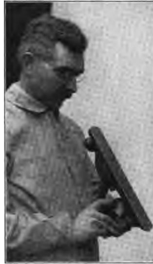
Fig. 26—Adjusting the Plane Iron
