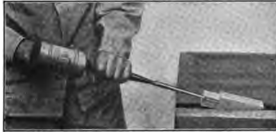
Fig. 67—Splitting Out Stock with Chisel
