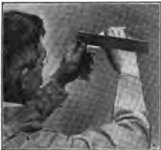
Fig. 67d—Testing Surface of Chisel Cut with Try Square
