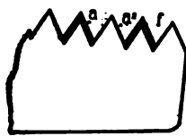
Fig. 4—Shape of Hand or Crosscut Saw Teeth
