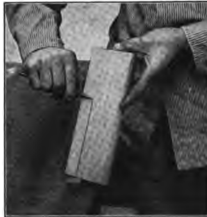
Fig. 128—Edge Lining for Round and Bevelled Edges
