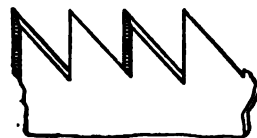
Fig. 143 a —Teeth Filed too Straight on Front Face
