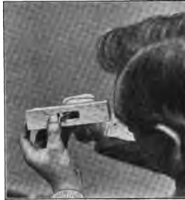
Fig. 70l—Chisel Used as Straight-Edge to Test Side of Mortise
