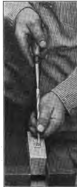
Fig. 70 g —Trimming Sides of Mortise with Chisel
