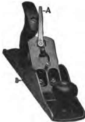
Fig. 24—Plane Stock, Bit and Clamping Iron Removed
