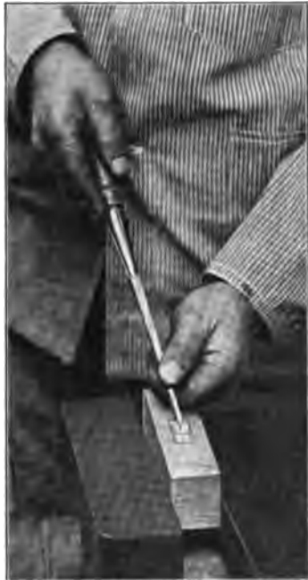
Fig. 70 f —Splitting the Chips with the Chisel
