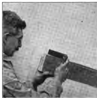
Fig. 30—Testing Edge for Squareness
