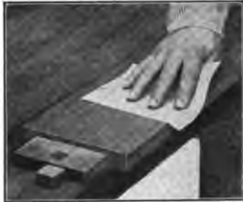
Fig. 178—Incorrect Way of Holding Sand-Paper
