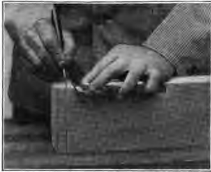
Fig. 39i—Putting Knife and Square in Position for Drawing Line on Edge
