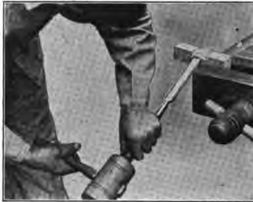
Fig. 68a—Removing Stock from Part II of Lap Joint
