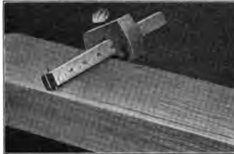
Fig. 35—Position of Gauge for Making a Line
