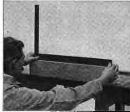
Fig. 29—Carpenter's Square Used as Straight-Edge
