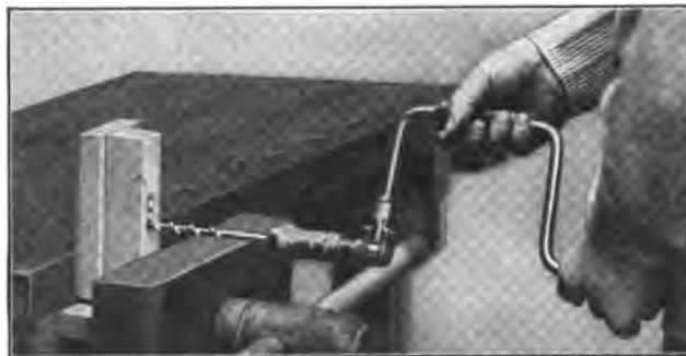
Fig. 71b—Boring into Block
