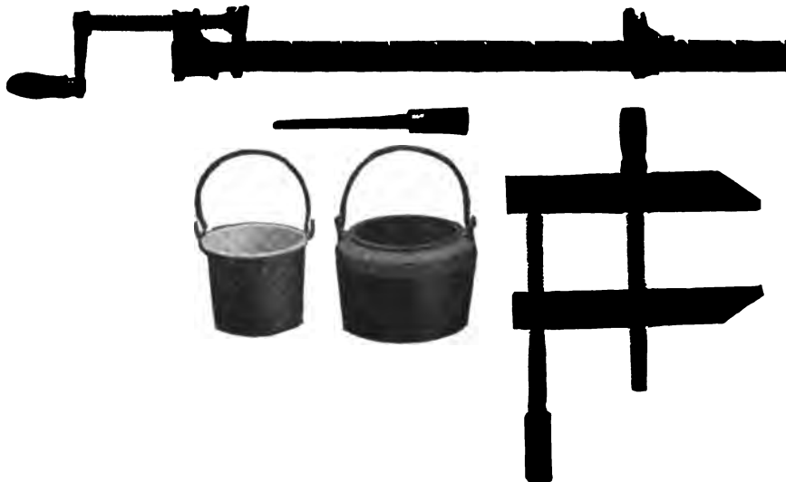
Fig. 123—Gluing Outfit. Photograph Showing Glue-Pot, Glue Brush, and Clamps
