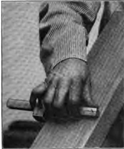
Fig. 36—Holding the Gauge for Making a Line
