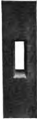
Fig. 70k—Sides and Ends of Mortise Pared to Lines with Centre High
