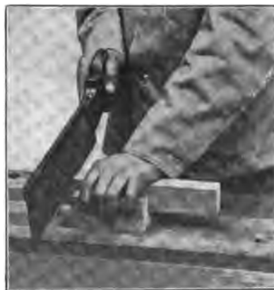
Fig. 66b—Cut Started. Position of Hand on Piece Changed
