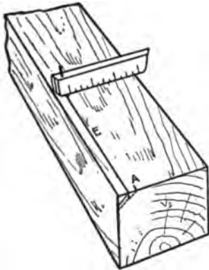
Fig. 127—Incorrect Method of Laying Out Bevelled and Round Edges
