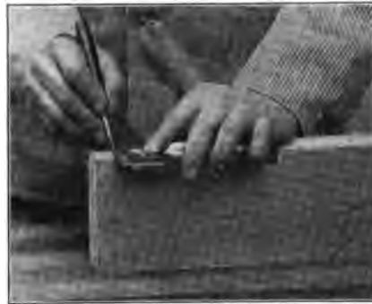
Fig. 39j—Knife and Square in Position for Drawing Line on Edge
