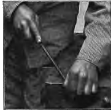
Fig. 176e—Turning Edge of Scraper with Butcher's Steel
