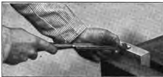
Fig. 69 c —Beveling Projecting End with Chisel
