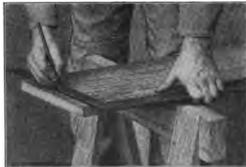
Fig. 1a—Cross Lining with Pencil and Carpenter's Square
