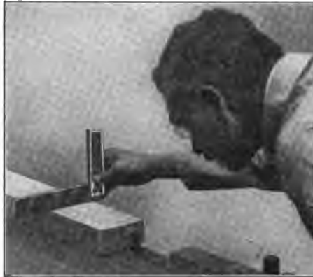
Fig. 28—Try Square Used as Straight-Edge
