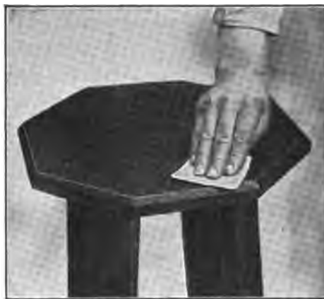
Fig. 182—Sand-Papering Stain or Varnish Coat
