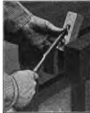
Fig. 70i—Bevelling to Side Lines of Mortise
