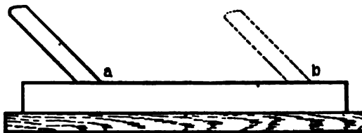
Fig. 18—Correct Method of Oil-Stoning Plane Bit
