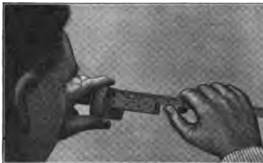
Fig. 34—Setting the Gauge to Exact Dimensions
