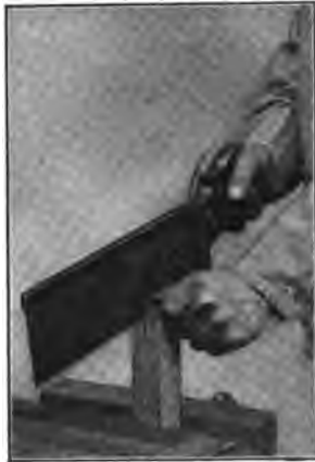
Fig. 67 a —Sawing Out Stock
