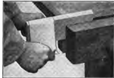
Fig. 181—Rounding an Edge with Sand-Paper
