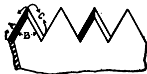
Fig. 143—Usual Shape of Saw Teeth for Crosscutting
