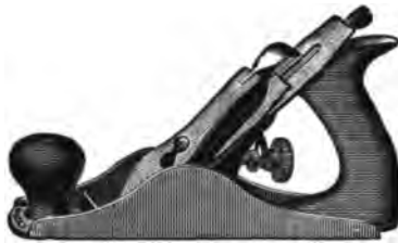
Fig. 7—Plane for Cutting with the Grain
