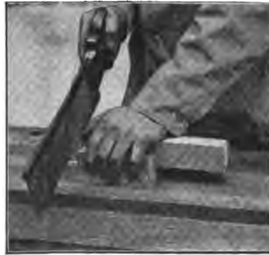
Fig. 66a—Hand and Saw in Position for Starting Saw Cut
