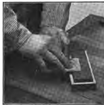
Fig. 176c—Oil-Stoning Flat Side of Scraper to Remove Feather-Edge
