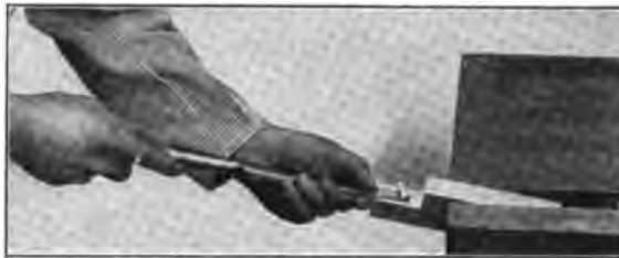
Fig. 67c—Paring Centre Down to Side Lines
