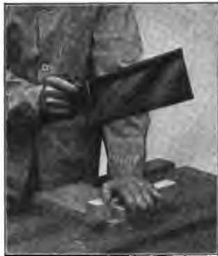
Fig. 66—Piece Placed on Bench Hook Ready for Sawing
