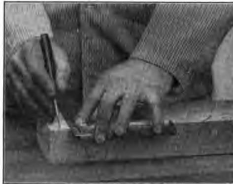
Fig. 39f—Putting Knife and Square in Position to Draw Line
