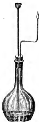
Students' apparatus for making arsenic spots.
