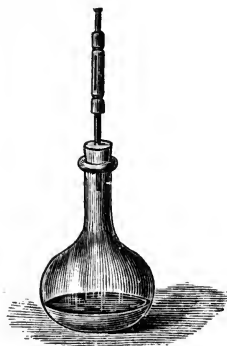
Flask for dissolving iron for volumetric determination.
