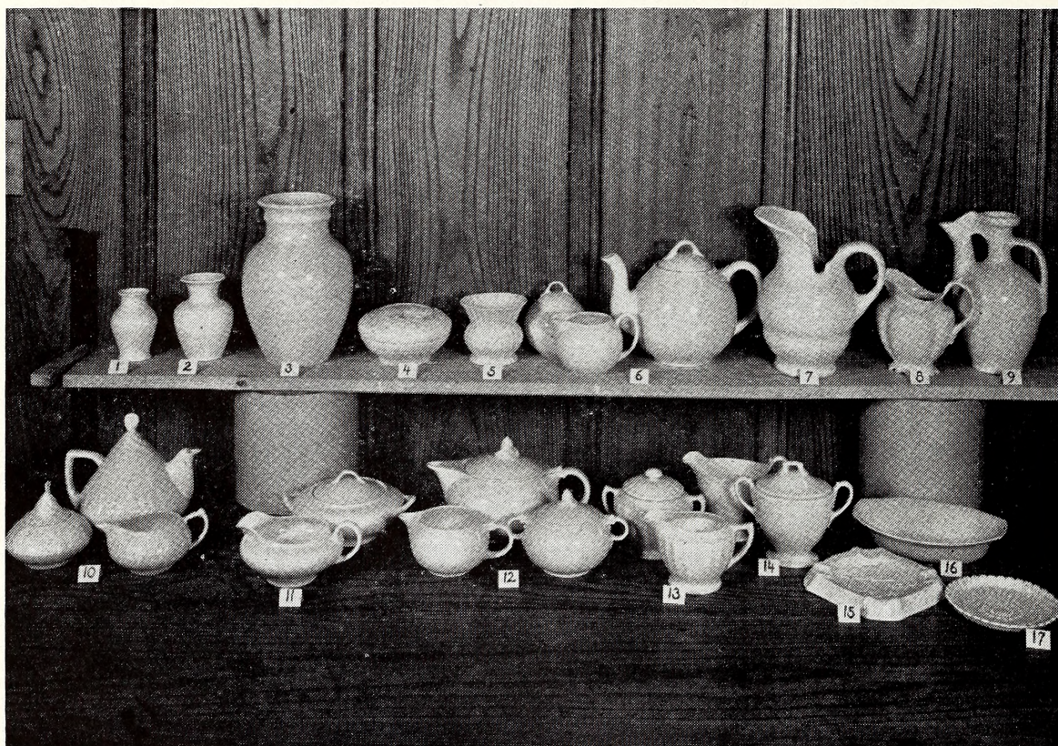
Figure 11. Test Ware Produced Experimentally at TVA Ceramic Laboratory. Made Exclusively of North Carolina Kaolins and Other Domestic Materials.
