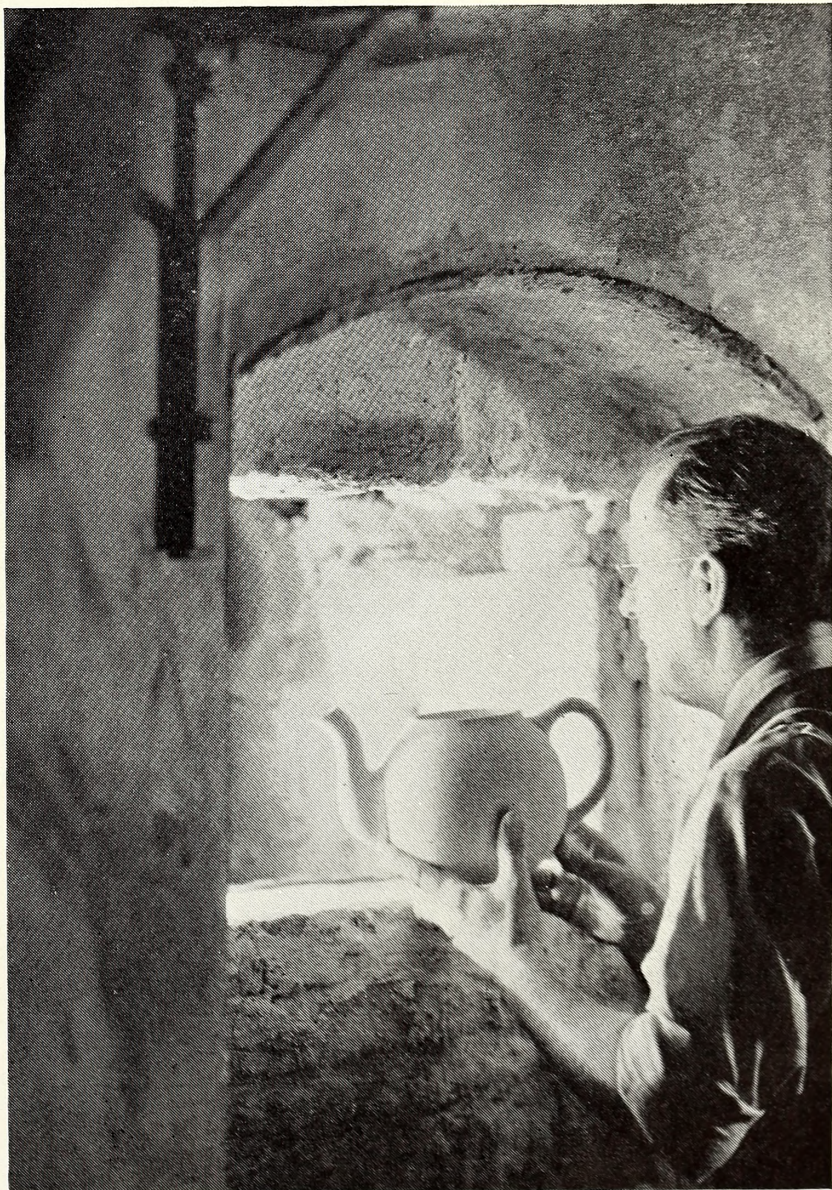
Figure 12. Test Ware Produced Experimentally at TVA Ceramic Laboratory. Made Exclusively of North Carolina Kaolins and Other Domestic Materials.
