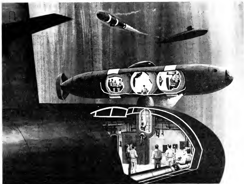
FIGURE 18.—Artist's sketch of planned U.S. Navy Rescue Vehicle evacuating crew from disabled submarine.
