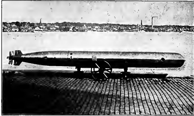
THE AUTOMOBILE TORPEDO, THE WEAPON USED BY DESTROYERS AND SUBMARINES
