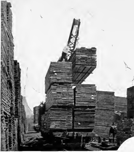
One of the Westwood Crane Crews Piling Lumber for Air-drying. One board at a Time is Too Slow. The Record for One Crane—10 Hours is 678,900 Feet, Board Measure.
